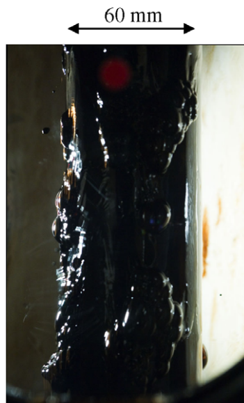
Fig. 1. Photograph of a black liquor falling film during evaporation. The photograph shows the evaporator tube (60-mm outer diameter) with black liquor falling film on the outside of the tube wall. The black liquor had a temperature of ~110 °C and the circulation flow was 5.56 \times 10^{-5} \text{ m}^3/\text{s} (Re number of ~600). The temperature difference between the heating steam and the evaporating black liquor film was ~8 °C. (The red dot in the top of the picture is a mark associated with the viewport glass. The lighter part to the right in the photograph is from the flash located inside the evaporator jacket.)
