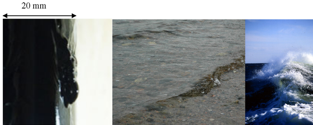
Fig. 3. The left photograph shows a black liquor falling film during evaporation for a low circulation flow where bubbles are created in a surge or wave front. The middle image shows wave-breaking and bubble formation on a beach; the right image shows wind-stress, wave-breaking at sea.
